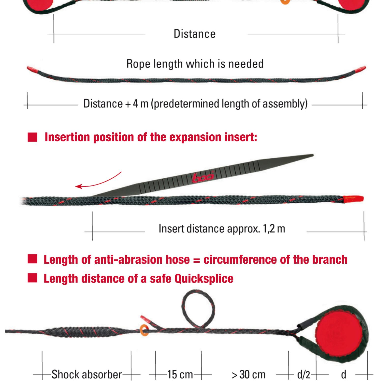
Insertion position of the shock absorber: arbitrarily on free distance of the rope
